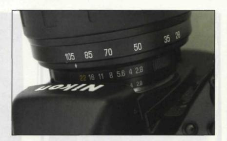
focal lengths, the effective f-stop increases. This increase in f-stop, requires you drop your shutter speed accordingly. This makes this type of zoom lens more difficult to use at the longer focal lengths.
